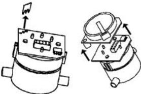
**!** Do not remove shorting jumpers/auxiliary circuit boards of the new measuring cells until immediately before installation. Do not leave the measuring cells without a shorting jumper/auxiliary circuit boards for longer than 15 min.
