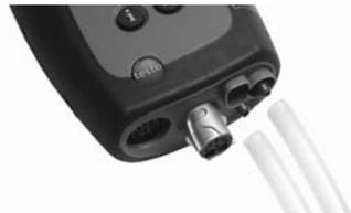
Pressure sockets p+ and p- can only be used with instruments offering the "Pressure/flow speed measurement" option.
