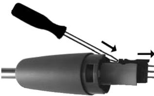
1 Release the probe catch by pressing the key on the probe handle and remove the probe module.
