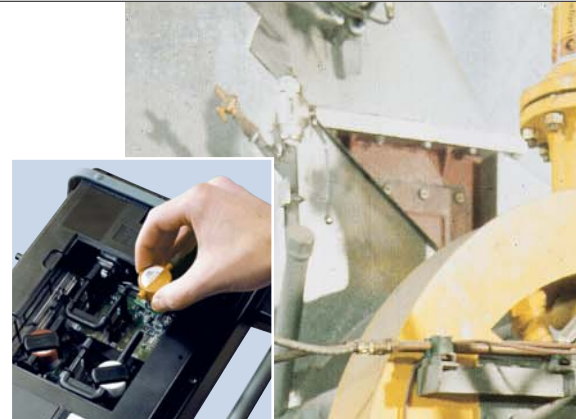
Measuring cells can be changed quickly and easily by the user on site
