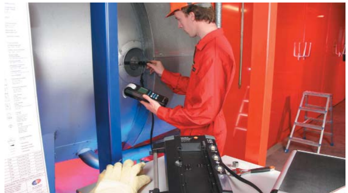
testo 350 XL: Portable measurements on turbines (O 2 , CO low , NO low , NO 2 )
