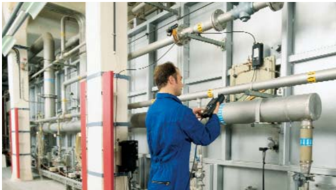
testo 350 S: Set for fast emission monitoring on industrial burners (O 2 , CO, NO)
