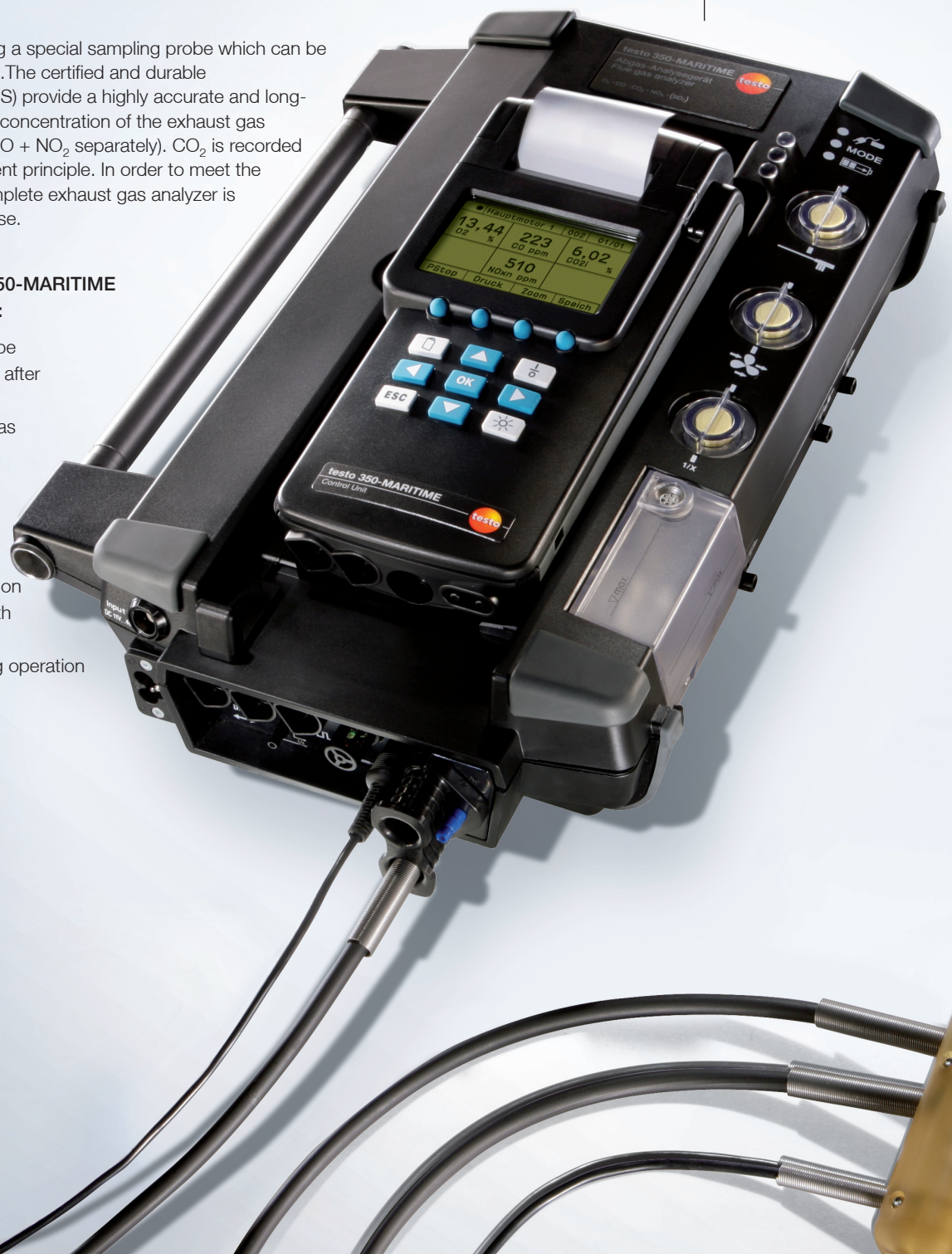
Emission analyzer testo 350-MARITIME
