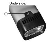
**E1:** Front bezel is not fastened correctly. If the E1 message appears, the instrument must be switched off. Remove the front bezel screw, reseat the reflector and tighten the front bezel screw (①).
